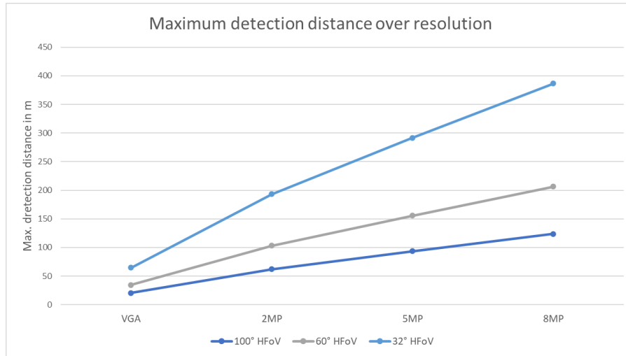
Figure 2.9: Maximum detection distance over camera resolutions of different horizontal field of views.
