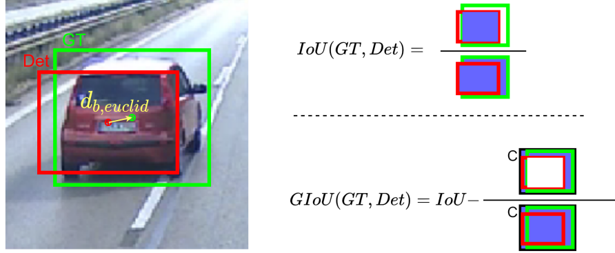
Figure 6.5: Proposed base distances in comparison for a 2D bounding box in image coordinates. Note, that these metrics can also be applied to other types of shapes and volumes, like OBBs.
