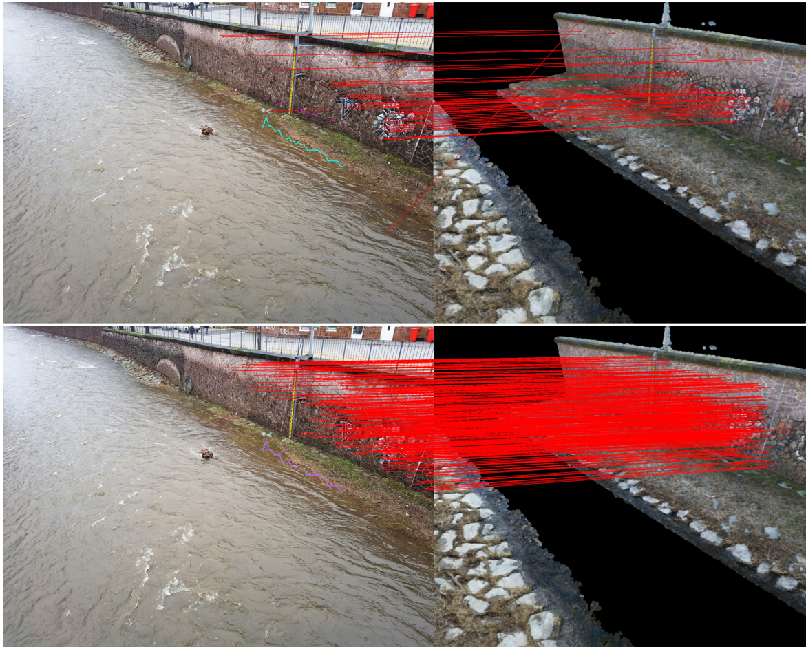
Figure (13.5): Comparison of real-to-synthetic image matching: SIFT+FLANN vs. D2-Net+BF. Top: SIFT+FLANN, 50 inlier matches still including false matches. Bottom: D2-Net+BF, 409 inlier matches. Blue line: image-measured 2D water line. Pink line: projected 3D water line.
