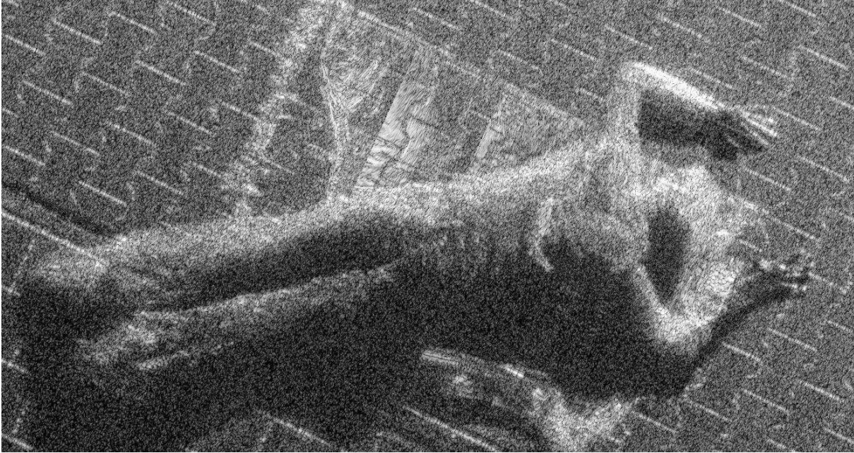
Figure 8.40: SAR image of the author at 300 GHz. Person is lying on the stomach with the head down on a blanket on paving stones. Through the transparent blanket, the pattern of the stones is visible. All fingers are clearly indicated.
