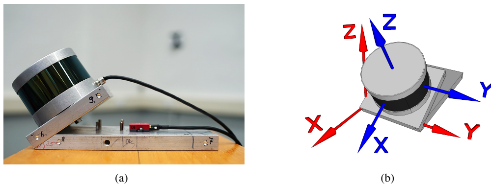
Figure 4.3: Laser scanner-based MSS with Velodyne Puck VLP-16 laser scanner and red Vectornav VN-200 IMU on a platform with numbered drilling holes (a) and schematic representation of the MSS with the red PCS and the blue SOCS of the laser scanner (b)
