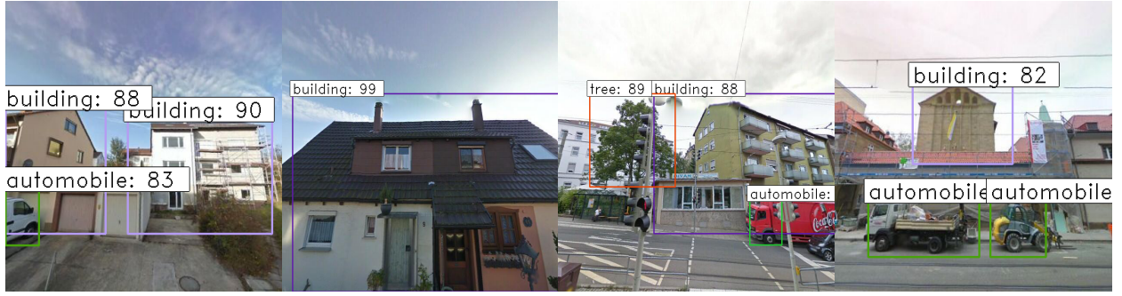
Figure 5.6: Faster R-CNN box detection results and associated probability for predicted class.
