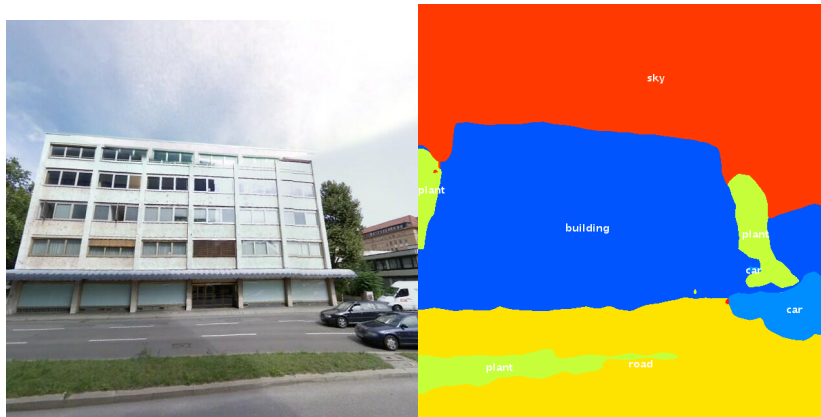
Figure 5.3: Input image and corresponding output from the FCN evaluation. The semantic class building is depicted in blue, sky in red, road in yellow, plant in green and car in bright blue, respectively.
