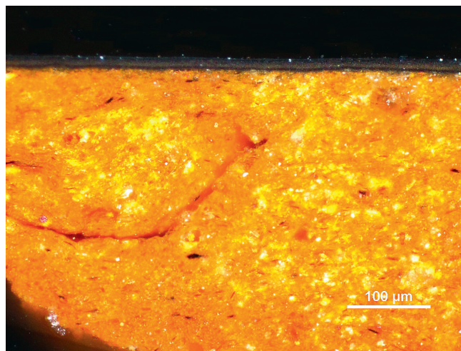
Fig. 11 Cross section of the black glaze taken on the internal side of the vase: 20x.
