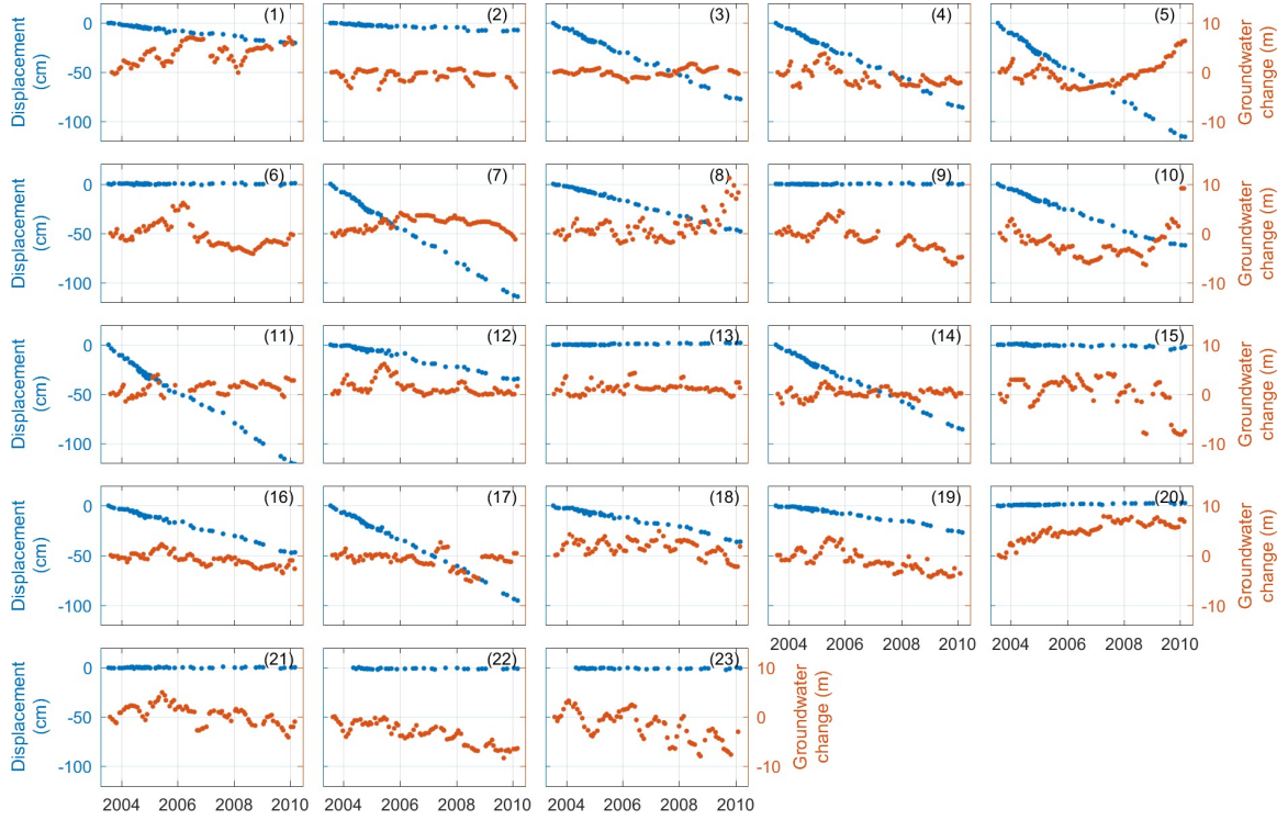
Figure 5.13.: Comparison of time series of vertical displacements and groundwater level changes at different locations. The numbers represent the measurement wells indicated in Figure 5.5-c. July 2003 is the reference date to estimate the groundwater variations.
