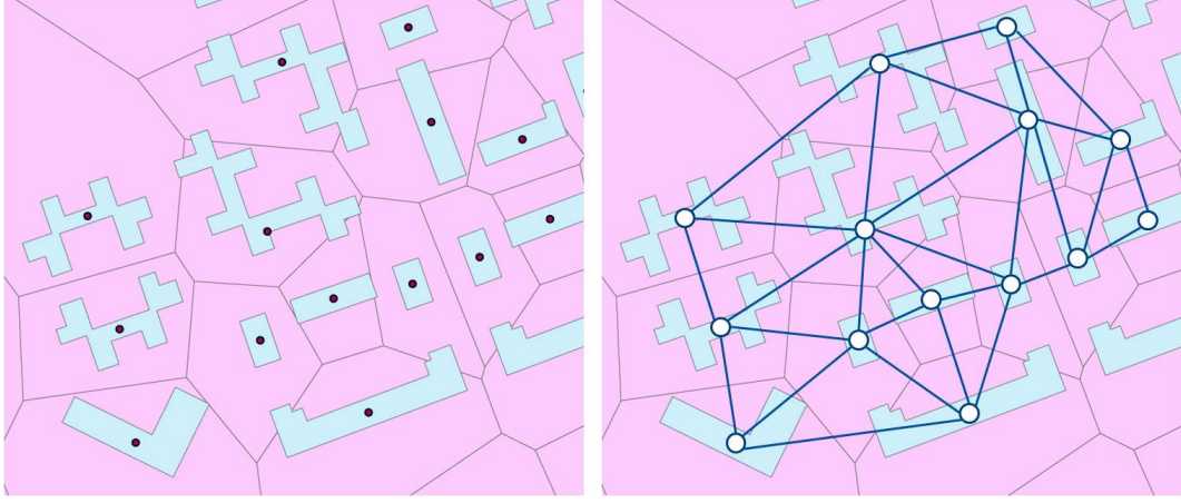
Figure 3.2: Definition of neighborhood of buildings: (left) polygons of buildings, their centroids marked with red points, and their Voronoi cells; (right) the MRF model with the edges connecting neighboring buildings
