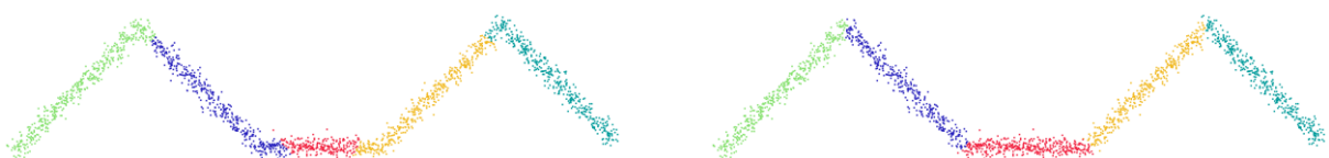
Figure 4.3. Segmentation results without (left) and with (right) reassignment of segment points; based on (Vosselman and Klein, 2010).
