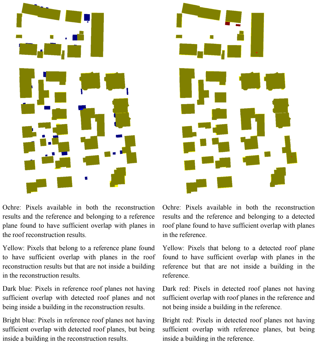
Figure 8.32. Evaluation result of the roof plane detection result once from the point of view of the reference (left) and once from the point of view of the result (right).
