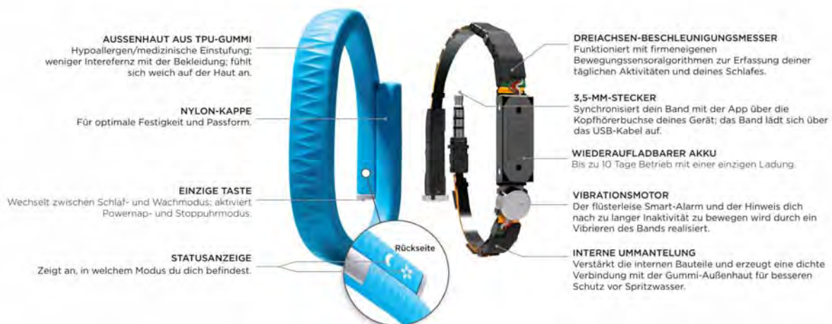
Abbildung 8.11 Jawbone UP – Komponenten (Jawbone 2014)
