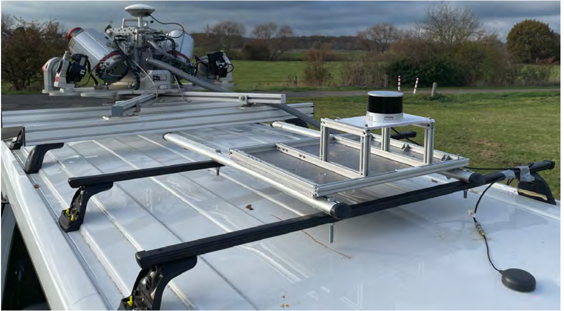
Figure 5.5.: Photo of the basic sensor setup: The Hesai PandarXT-32 is mounted on a platform at the front of the roof, and the RIEGL MMS is mounted at the end of the roof.
