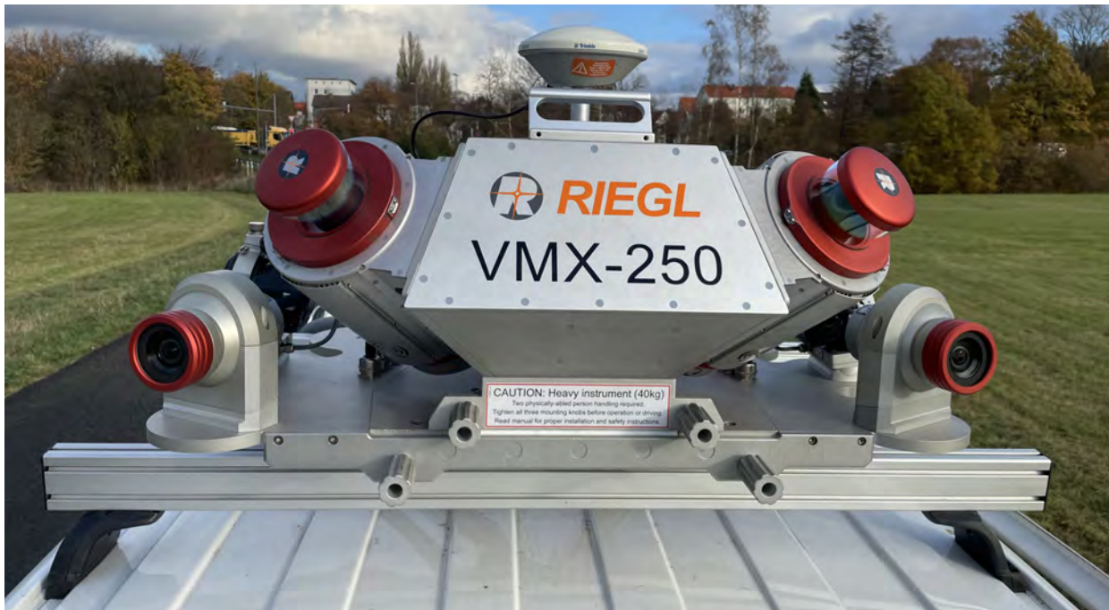
Figure 2.11.: RIEGL VMX-250 mobile mapping system mounted on the roof of a Volkswagen T5 minibus. The system comprises two RIEGL VQ-250 lasers scanners, four cameras, an Applanix POS LV GNSS/IMU system, an odometer attached to a wheel, and a control unit for operation, processing, and storage (RIEGL Laser Measurement Systems GmbH, 2012).
