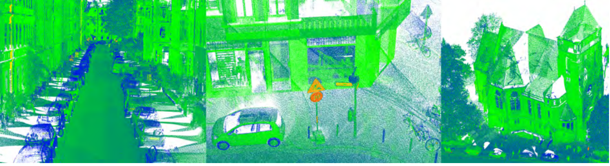
Figure 5.3.: Sections of the map point cloud from the Nordstadt data set. The points are colored according to the measured reflectivity value.
