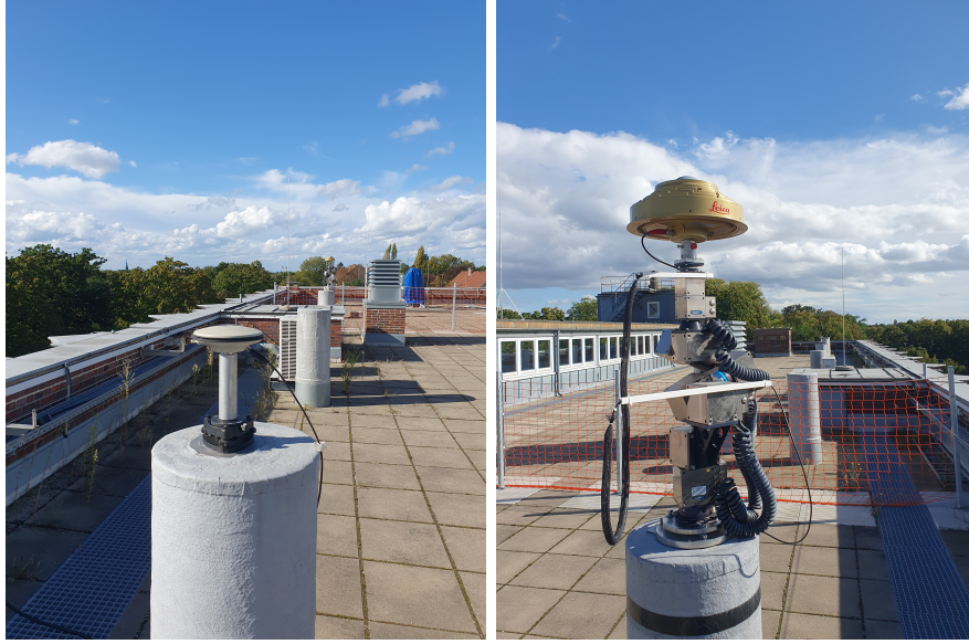
Figure 6.24: Measurement configuration for validation with category 2 antenna on pillar MSD4 (left) and category 1 antenna mounted on the robot (right).
