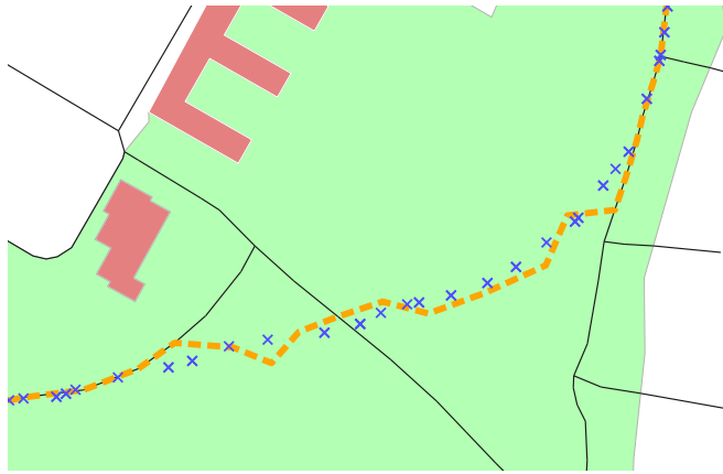
Figure 4.1: Example of a map with an embedded road network as well as free spaces and obstacles. The blue measurement-based trajectory is best explained by movement along the orange dashed path, which follows roads and free spaces where possible but contains no obstacle intersections.
