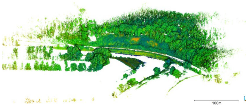
Figure 7: Terrestrial laser scan of the Freiburger Mulde (reflectance colored).
