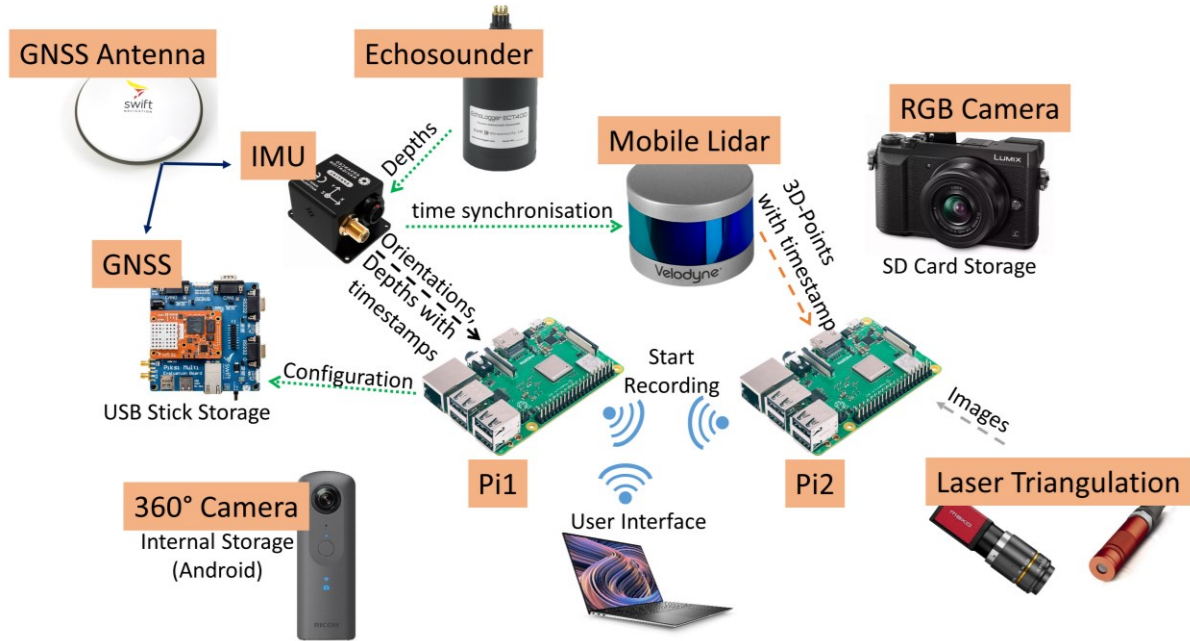
Fig. 2.3: Sensor configuration and system architecture of the multisensory system. The arrow colours indicate different types of connection: dark blue: antenna cable, green: serial port, black: USB, orange: Ethernet, grey: Ethernet (not yet included in the system). The light blue waves indicate a WIFI connection.
