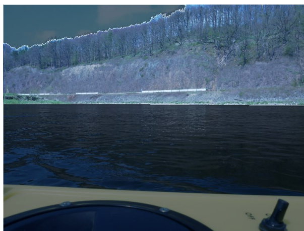
Figure 12: Measurement image used for SfM. Large areas of the image (sky and water) are not suited for matching and therefore masked-out.
