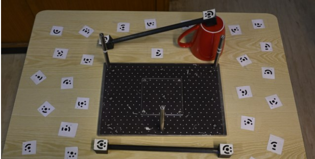
Figure 8: Measurement object consisting of ground plate and measurement panel.
