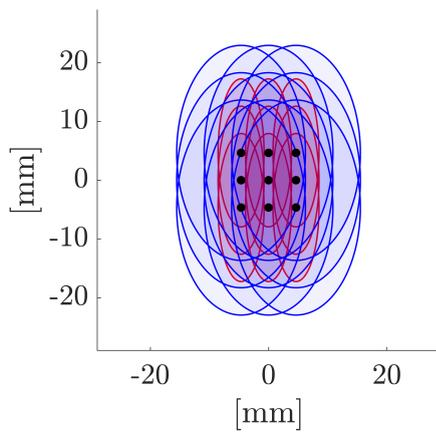
**Abbildung 5.11:** Comparison of the correlation lengths determined for the the Imager 5016 with empirical approach using the stochastic part of the point cloud (red) to the approach using the resolution capability (blue).
