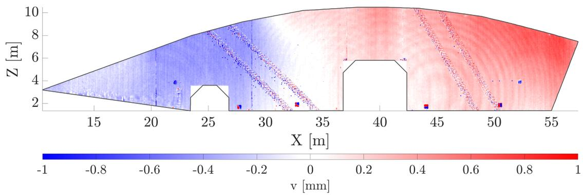
**Abbildung 5.20:** M3C2 differences between the two averaged point clouds of August and September using all calibrated scans of the Leica ScanStation P50 and the Z+F Imager 5016 (modified from Jost et al. [2023a]).
