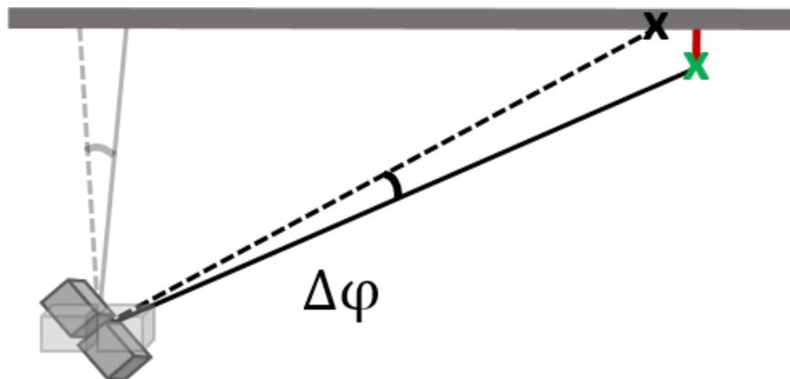
Abbildung 6.5: Impact of an erroneous horizontal angle on the point cloud comparison.
