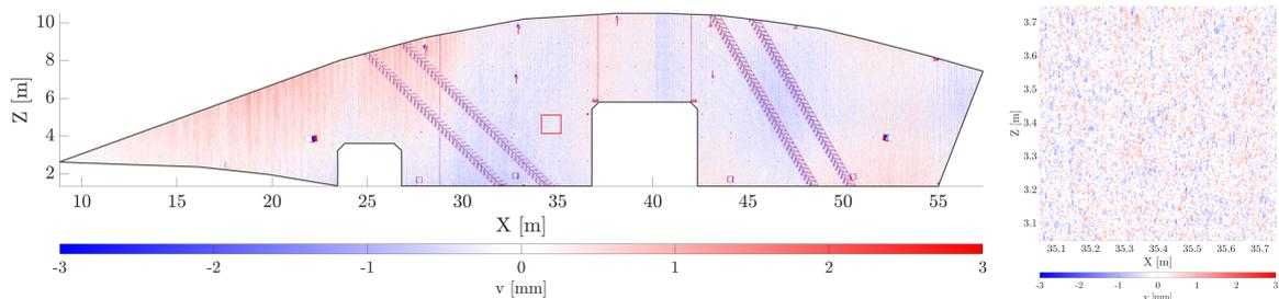
**Abbildung 5.19:** Stochastic part of the point cloud acquired with the Z+F Imager 5016 by illustrating the C2M distance between the reference point cloud and a calibrated scan from S6 (modified from Jost et al. [2023b]).
