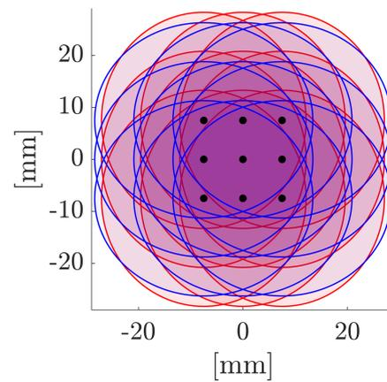
**Abbildung 5.12:** Comparison of the correlation lengths determined for the the BLK360 with empirical approach using the stochastic part of the point cloud (red) to the approach using the resolution capability (blue).
