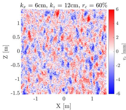
**Abbildung 5.5:** Simulated example for the stochastic part of correlated TLS measurements.
