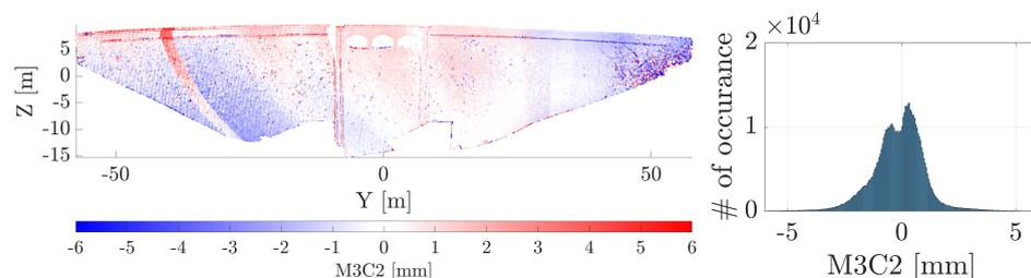
**Abbildung 3.7:** M3C2 differences between a scan of the Leica ScanStation P50 and the Z+F Imager 5016 that have been acquired within a short time from the same station. User calibration is applied to both scans.
