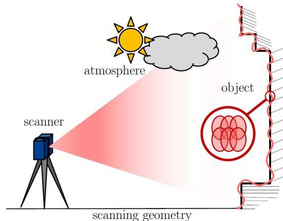
**Abbildung 3.5:** Error sources of terrestrial laser scans.
