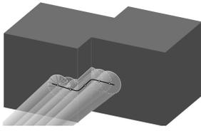
**Abbildung 3.3:** Overlapping laser spots on an object's edge.
