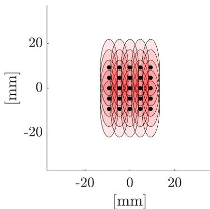
**Abbildung 5.9:** Exemplary representation of the correlation of 5x5 points measured with the Imager 5016. The black dots represent the measured points and the ellipses the area where the correlation is at least 37%. The axes of the ellipses correspond to the correlation lengths given in Tab. 5.2.
