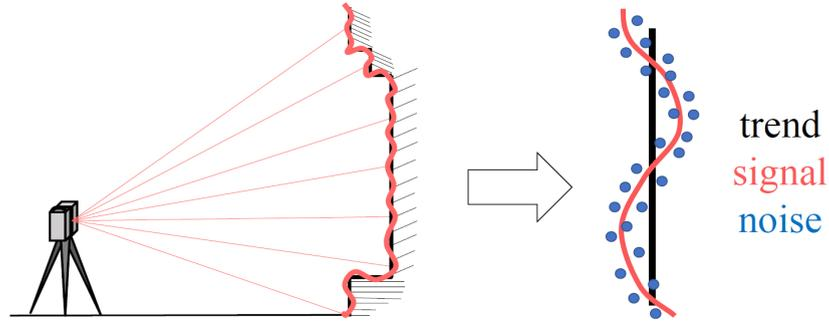
Abbildung 3.1: Composition of a TLS measurement: trend, signal, and noise.
