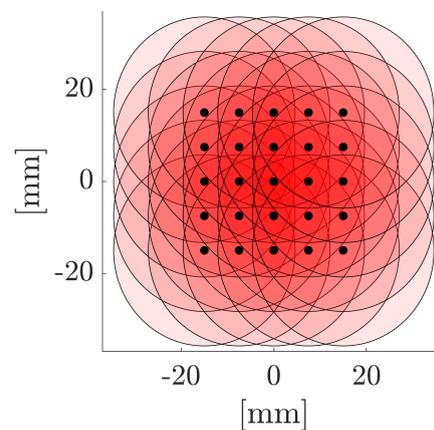
**Abbildung 5.10:** Exemplary representation of the correlation of 5x5 points measured with the BLK360. The black dots represent the measured points and the ellipses the area where the correlation is at least 37%. The axes of the ellipses correspond to the correlation lengths given in Tab. 5.2.
