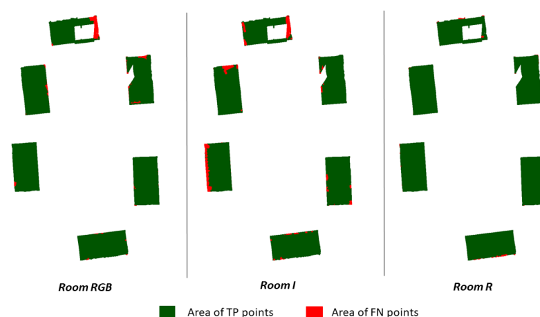
Figure 13. TP and FN areas of dataset Room at different semantic segmentations for the table class.
