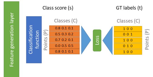
FIGURE 15. Process of feature extraction, classification and loss calculation at PointNet. Prediction class score ( s ) and ground truth label target ( t ) vector as one-hot encrypted matrix.
