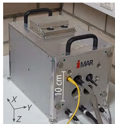
(b) The IMU encased in the iTempStab-AddOn
