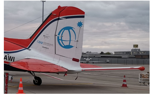
Figure 6.33: Magnetometer installed in the tail rod of Polar 5
