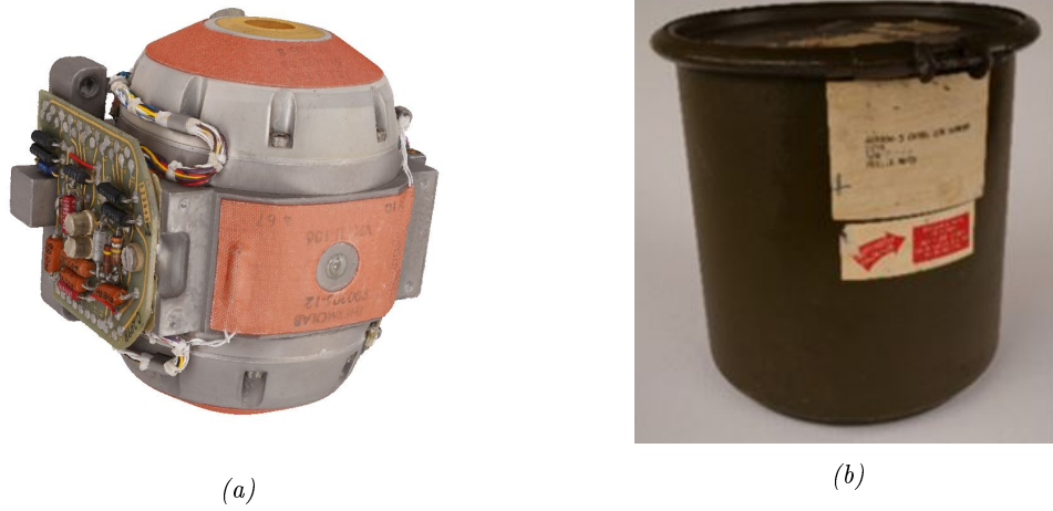
Figure 7.4: The Gyro G200 of the LN3 Inertial Platform: (a) Gyro G200; (b) G200 transportation box.
