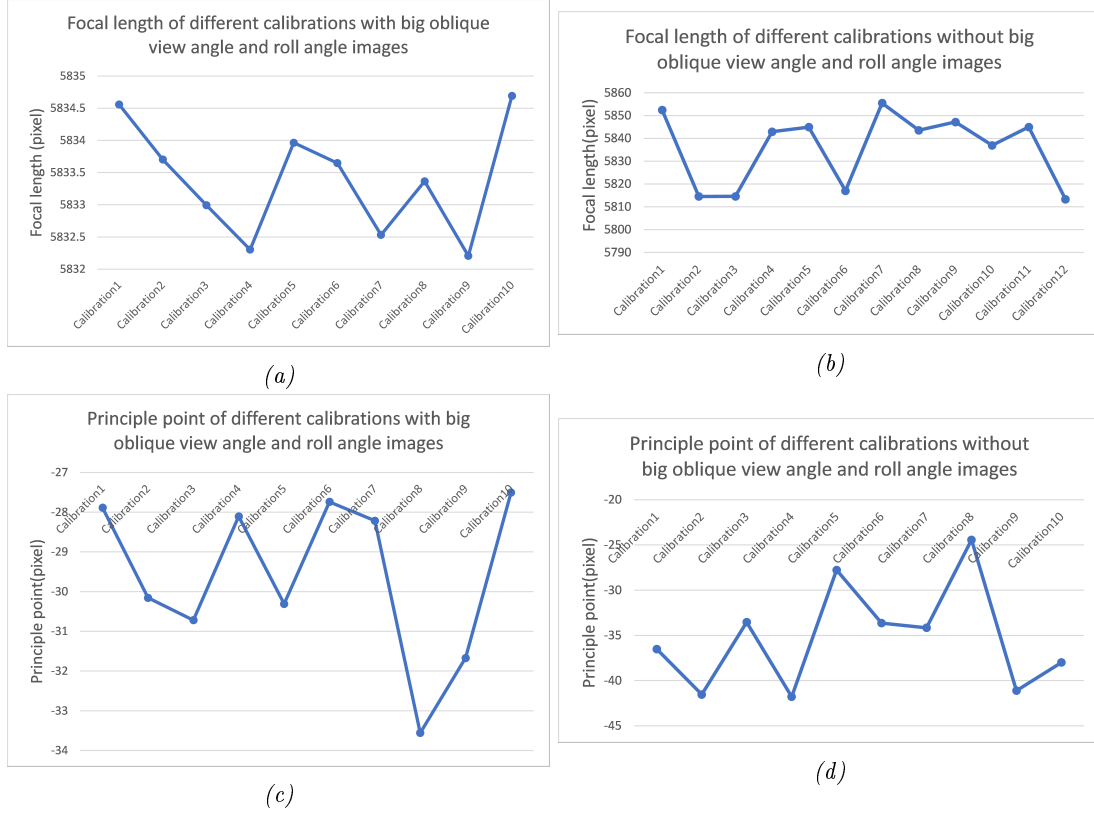
Figure 3.10: Temporal stability variation experiment results: (a) focal length of different calibrations with strong image block configuration; (b) focal length of different calibrations without strong image block configuration; (c) principle point of different calibrations with strong image block configuration; (d) principle point in X direction of different calibrations without strong image block configuration.
