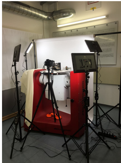
Figure 4.4: Photogrammetry turn-table setup.
