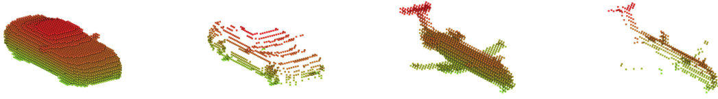
Figure 6.12: Examples of self-occluded and voxelized objects from the Shapenet dataset. Left: A complete car and the result of the simulated self-occlusion. Right: A plane and its self-occluded counterpart. All voxels are colored by height, where green is low and red is high.
