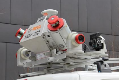
(a) The RIEGL VMX-250 Mobile Mapping System equipped with two line scanners
