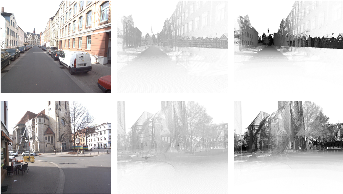
Figure 6.7: Each row shows the same scene. The images on the left show the real camera images. The images in the middle show the projected point cloud colored by reflectance and the images on the right are colored by the distance.
