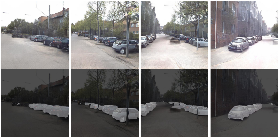
Figure 8.6: Cars successfully classified in synthetic images (bright grey) using Deepblabv3+ pretrained on PASCAL VOC.
