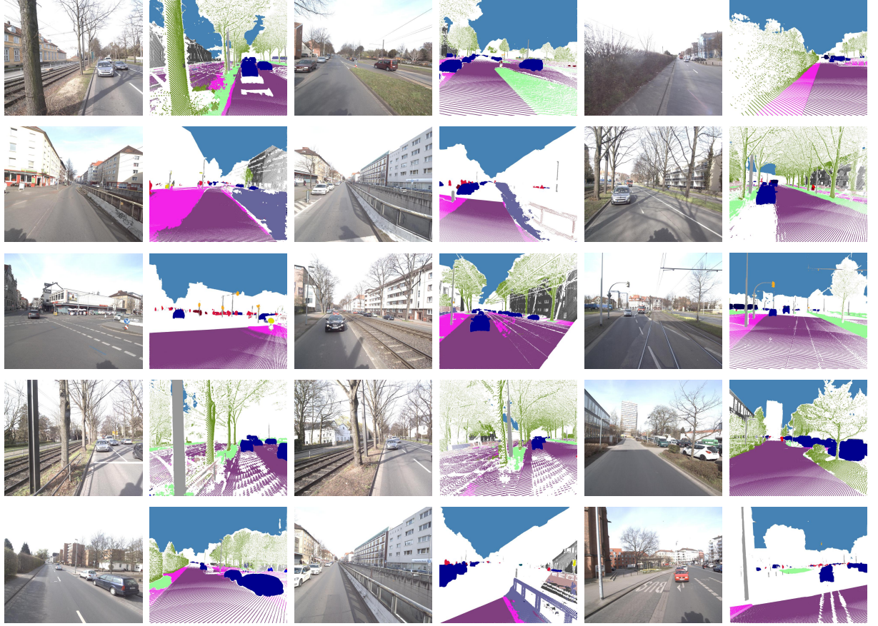
Figure 7.24: Randomly sampled pairs of images and labelled images created by MVNet using the merge strategy from Equation 7.10. The RGB images show the input data and the images to the right shows the predictions by MVNet which are used as pseudo labels for fine-tuning of Deeplabv3+.
