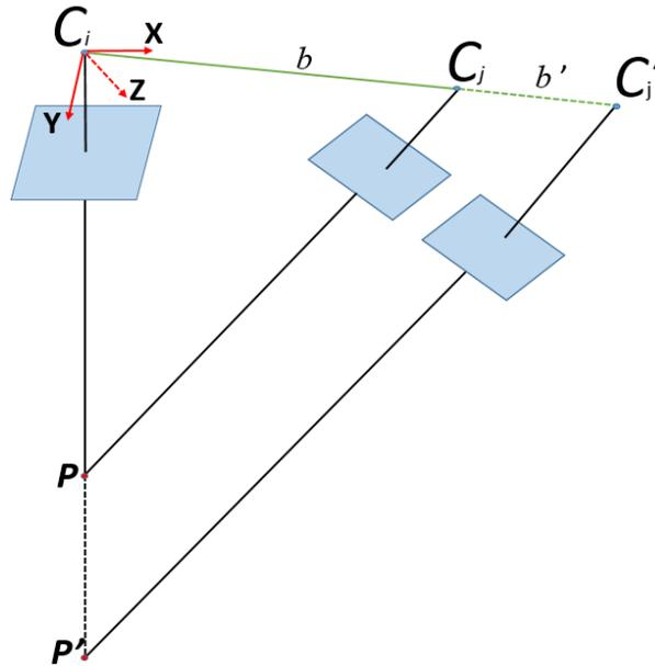
Figure 4.1: Local pairwise triangulation.  $\mathbf{C}_j$ : projection center of image  $j$  if the length of the baseline is defined as  $b$ .  $\mathbf{P}$ : the position of a tie point under these circumstances.  $\mathbf{C}_j'$ ,  $\mathbf{P}'$ : Projection center of image  $j$  and tie point if the length of the baseline is changed to be  $b'$ .
