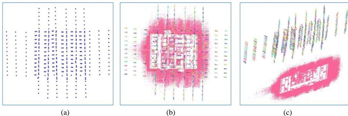
Figure 6.13: Visualization of the result after bundle adjustment. (a) is the exposure positions from the provided reference. (b) and (c) are the reconstruction results of PM\_GTC\_IO observed from two various perspectives.
