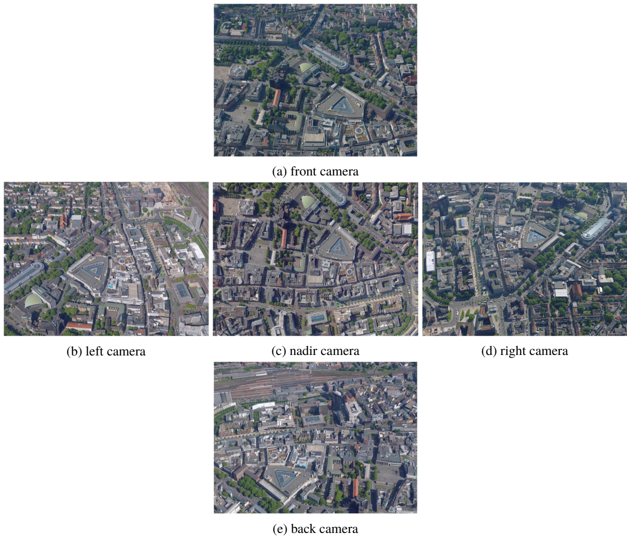
Figure 5.6.: Five exemplary images taken from different views in one small oblique aerial image block (block4). Images (a), (b), (c), (d), (e) are taken by front, left, nadir, right and back camera, respectively. As those five images come from different imaging stations, there is a large viewpoint and viewing direction change among any two of the images taken by different cameras.
