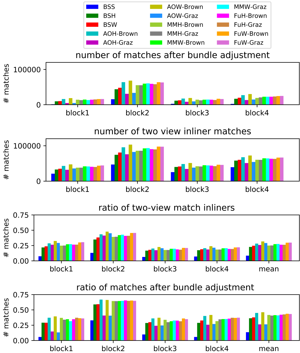
Figure 5.18.: Number and ratio of matches for different blocks. From top to bottom: number of matches after bundle adjustment ( N_{match}^{surv\_BA} ), number of two view inlier matches ( N_{match}^{inl\_2view} ), ratio of two-view inlier matches ( R_{initial}^{inl\_2view} ) and ratio of matches after bundle adjustment ( R_{surv\_BA}^{inl\_2view} ). All four of the bar figures share the same label for different variants, as shown in the top figure. For the two related ratios (3rd and 4th row), the mean values over the four groups are also provided at the end of each bar figure.
