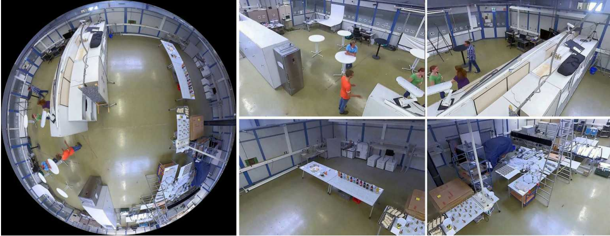
Figure 4.5: Illustration of a general de-warping result where one fisheye image was de-warped to four central projection images. Left: fisheye reference frame. Right: reference frame is de-warped to four central projection images (south-west, north-west, north-east, south-east).
