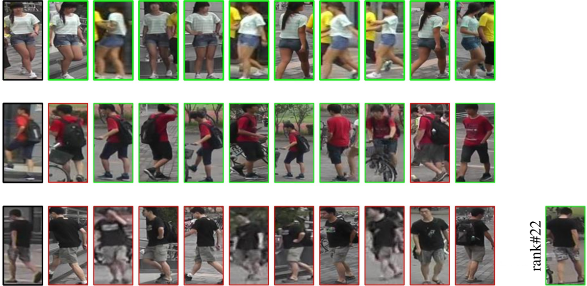
Figure 2.3: PRID as retrieval task: three unknown persons (probes) are requested (one per row). Probes (left), are bordered by black bounding boxes. From left to right, the ten most probable matches are depicted (rank#1 - rank#10) with decreasing similarity. Correct matches are displayed in green bounding boxes, false matches in red bounding boxes. The first row shows a very good result. All the top ten matches are correct. The second row shows an example where the first and ninth match are wrong. The third row shows an example where all ten matches are wrong, and the correct match is on rank#22. Cropped images of persons are taken from the Market-1501 dataset [Zheng et al., 2015a].
