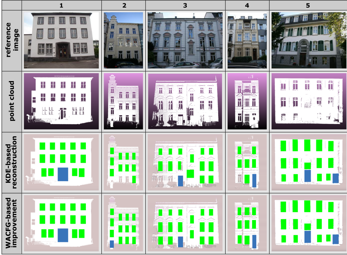
Figure 3.8: Façades reconstructed with the WACFG. Windows are colored in green and doors in blue. The first row shows reference façade images. The second row depicts the corresponding input 3D point clouds. Row three represents a kernel density-based reconstruction of each façade. Deficiencies of the kernel density estimation are overcome using the WACFG model.
