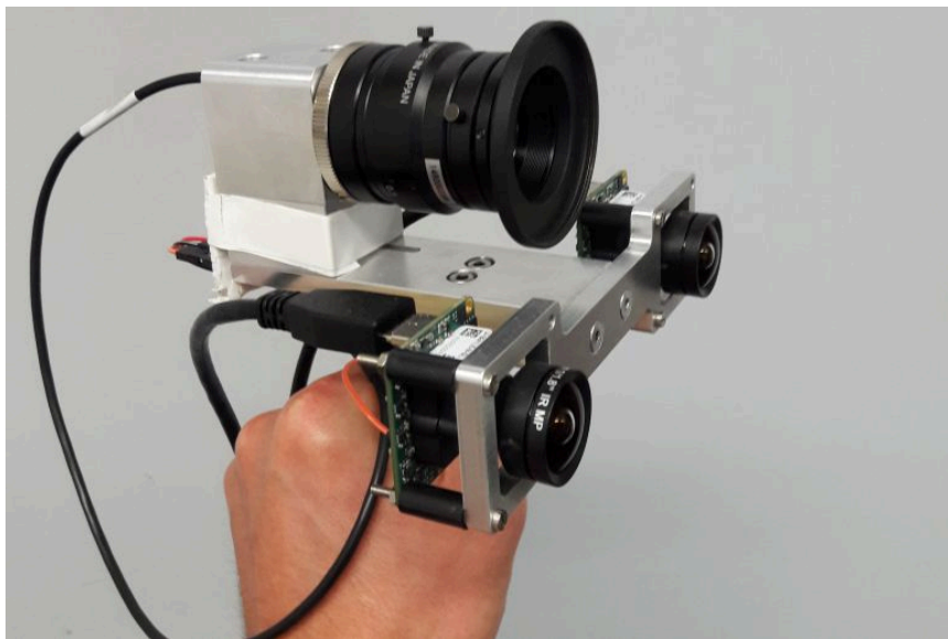
Figure 10.1: Handheld platform to acquire time synchronized image sequences from a focused plenoptic camera and a stereo camera system.
