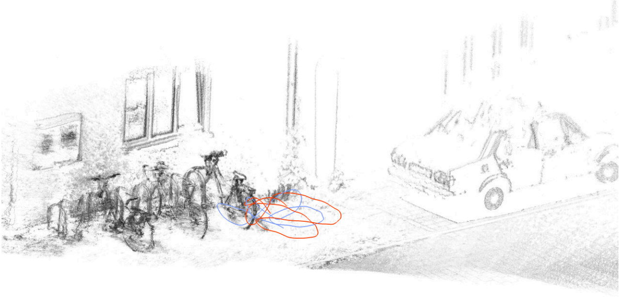
Figure 10.5: Semi-dense point cloud generated by DPO overlaid with the loop closure trajectory of the start and end segment, used as ground truth, and obtained from SfM on the stereo images. Start segment of the trajectory is marked in red and the end segment in blue.
