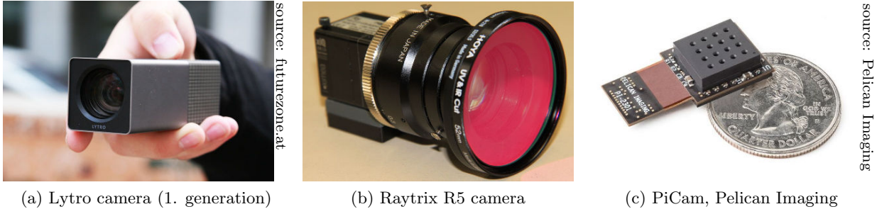
Figure 1.1: Different light field sensors. While (a) and (b) are both micro lens array based plenoptic cameras, (c) is a miniaturized 4 \times 4 camera array.
