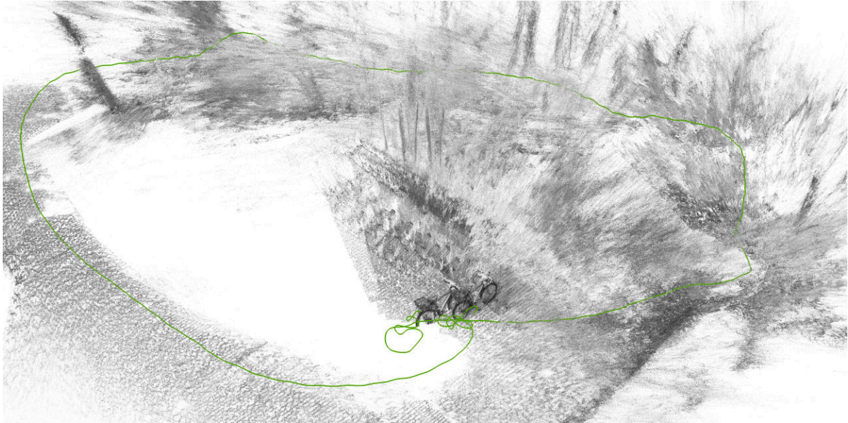
Figure 10.16: Complete trajectory and point cloud calculated by DPO for a scene with abundant vegetation (sequence #3). Even though the point cloud looks quite random, the camera trajectory, which has a length of approximately 80 meters, was estimated accurately.
