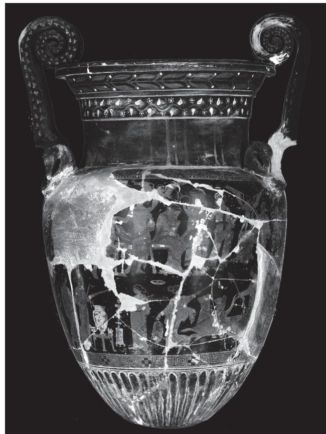
*Fig. 9 UV image of krater (F 3257) showing fluorescence of 19<sup>th</sup> century interventions.*
