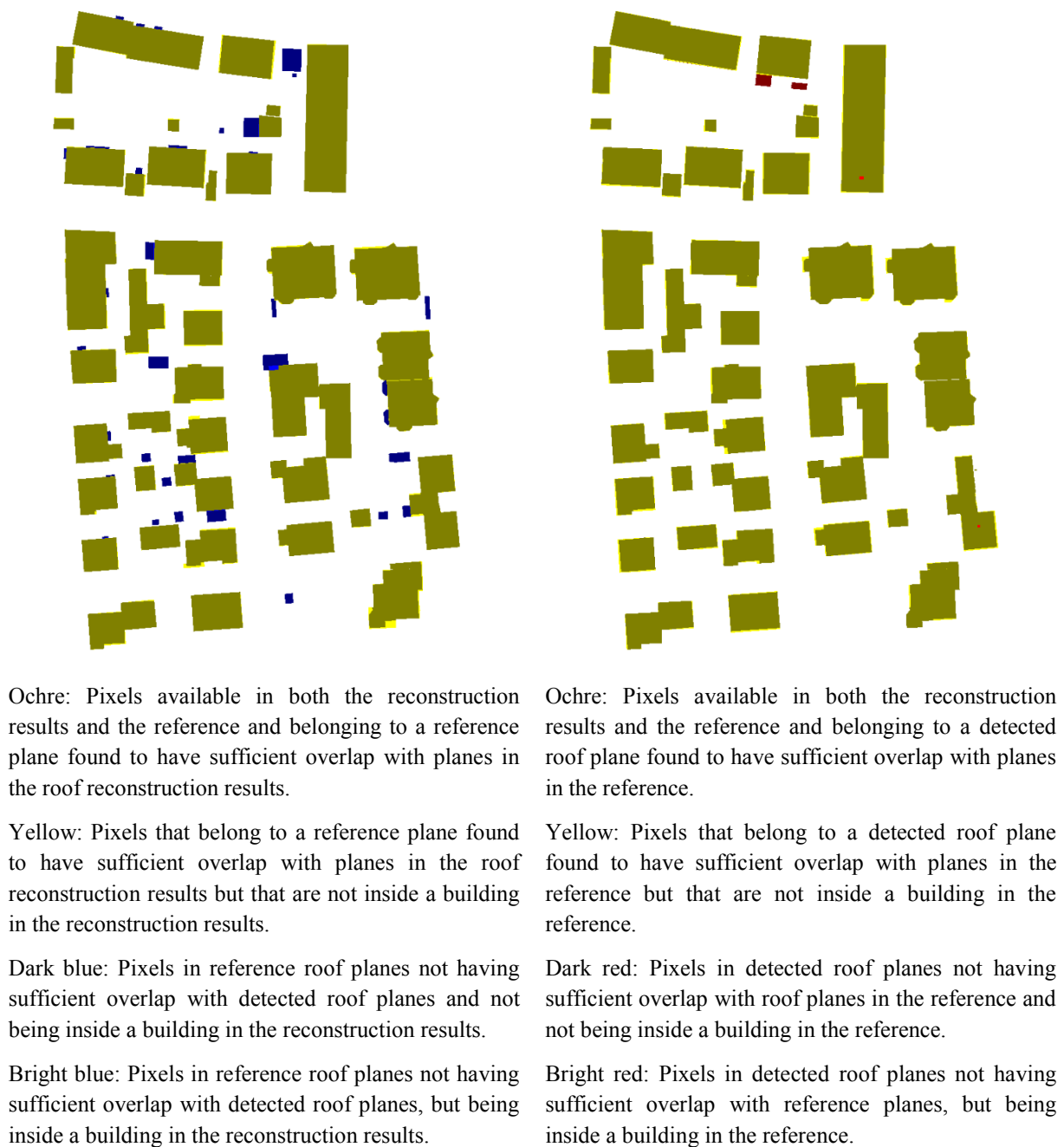
Figure 8.32. Evaluation result of the roof plane detection result once from the point of view of the reference (left) and once from the point of view of the result (right).
