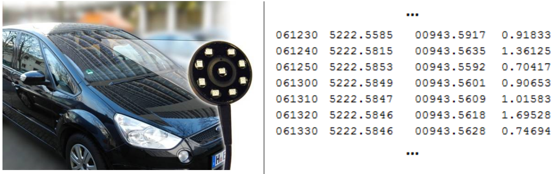
Figure 5.2: Left: The Xanonex optical rain sensor, which is placed behind the windscreen (image courtesy of B.Heinrich, Institute of Hydrology, Leibniz University Hanover). Right: Extract of raw ASCII data with time in UTC (first column from left), WGS84 latitude (second column), WGS84 longitude (third column) and the sensor reading in the unit [s/10s] (fourth column).
