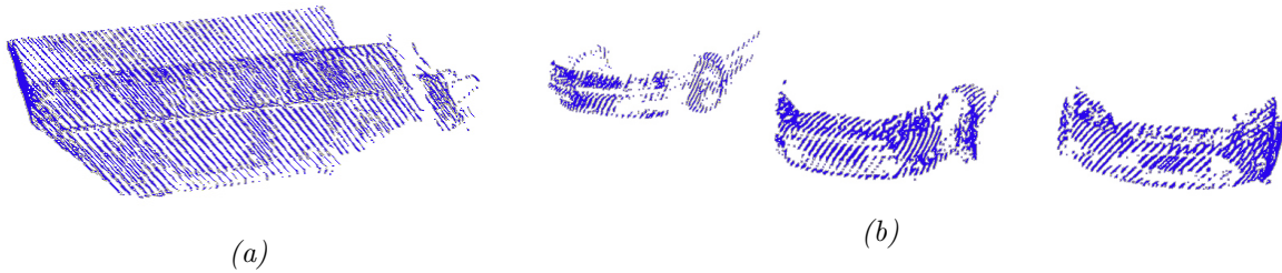
Figure 4.9: Examples for a false positive (construction trailer in (a)) and false negatives (vehicles parking perpendicular to the lane in (b)).
