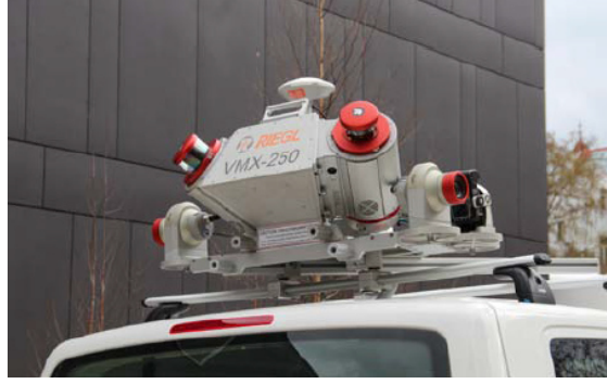
Figure 4.1: Riegl VMX-250 mobile mapping system with two 2D laser scanners, four cameras, and a global navigation satellite system (GNSS) receiver.
