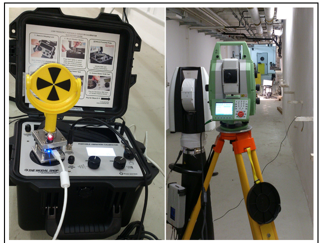
Figure 7. Vibration analysis of a controlled excitation based on acceleration measurements from the PSVC 9210D, video streams from the telescope camera of the Leica MS50, 3D coordinates from the LT Leica AT960-LR and acceleration measurements from the IMU Brick 2.0.
