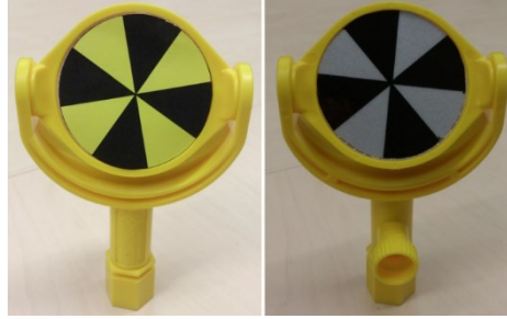
Figure 9. Designed circular target with line pattern: (left) paper printed target and (right) target printed on reflective tape.
