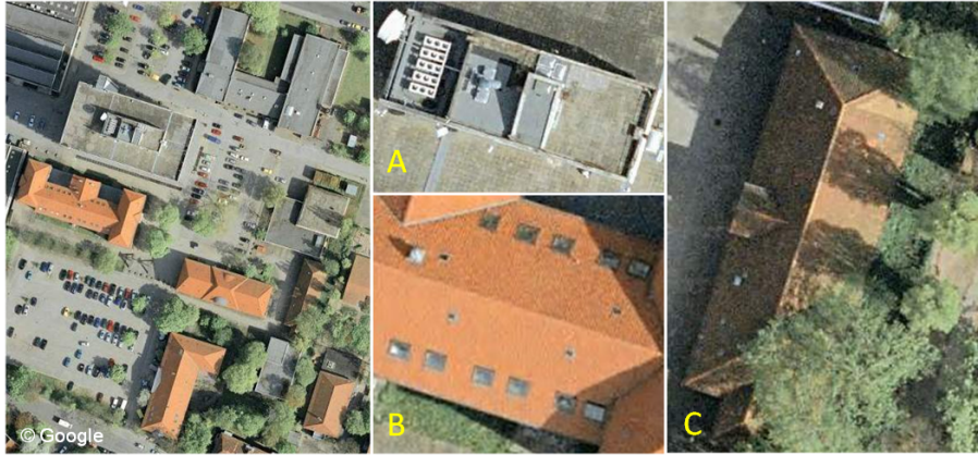
Figure 2.1: Causes of laserscanning data artefacts in urban areas (left): Complex roof structures (A), reflections (B), and occlusion (C)
