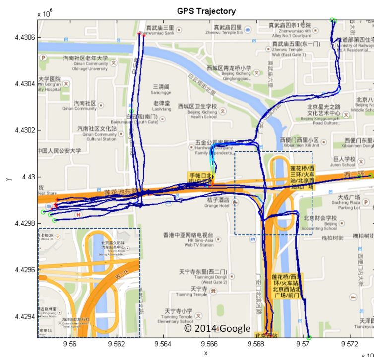
Figure 4.6: Collective behaviors in the case of a turn restriction: Trajectories passing the road intersection from the bottom to the left show a collective detour and indicate a turn restriction, which is proven by the street map.
